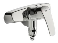
Utility room faucet. Wall-mounted utility room faucet with quick release coupling for ø13 mm hose and vacuum breaker. There are also in-built limitation options for water temperature and maximum flow-rate.
