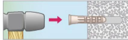
2. Knock in the Lightweight concrete plug with the help of a hammer in the lightweight concrete. Knock the plug in until it is flush with the surface of the substrate.
