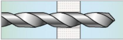
1. Drill the hole according to Technical data below. Be careful not to damage the drywall on the back and around the exit hole.
