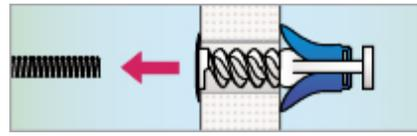
3. Pull the screw carefully and check that the wings have gripped at the rear. Unscrew the screw.
