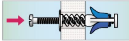
2. Press the Duo-Max through the board with help of the screw.
