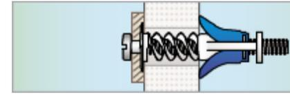
4. Mount the object. The installation is finished.
