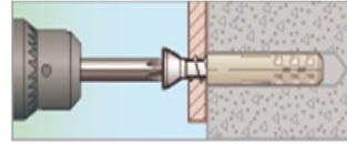
3. Mount the detail using an appropriate screw. The screw must go through the plug by about 3-5mm.
