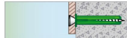
1. Drill the hole according to Technical data below.
