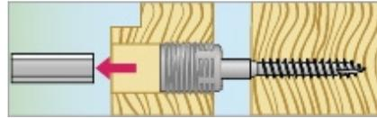
2. Use Frame screw tool UN-T or KMN, use the same tools for adjusting.
