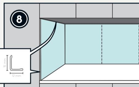
L-Profiles can be used on all cut surfaces to hide screws.
