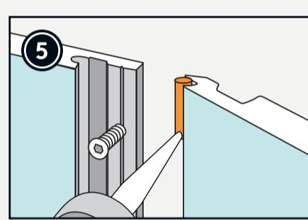
Fasten first panel with Fibo Screws. Apply sealant on the left side of next panel before connecting for a waterproof result.
