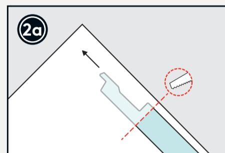
Trim the locking part from the first panel, ensuring to leave 2-3 mm space for the L-profile if this is chosen.
