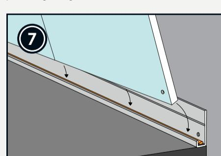
Apply sealant to the base of the bottom profile. Lift the panels collectively and place in the bottom profile. Remove excess sealant.
