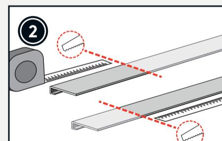
Adjust length of bottom profiles. Place a string of Fibo Seal under the bottom list for a waterproof system.
