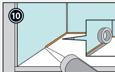
Apply Fibo Seal in the gap between the panels and worktop, and in corners. Masking tape on worktop can be used. Use Fibo Clean and Fibo Sealing Tools for a nice end result.
