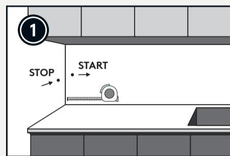
The panels are installed from left to right. Adjust the height of the panels in relation to any wall cabinets.
