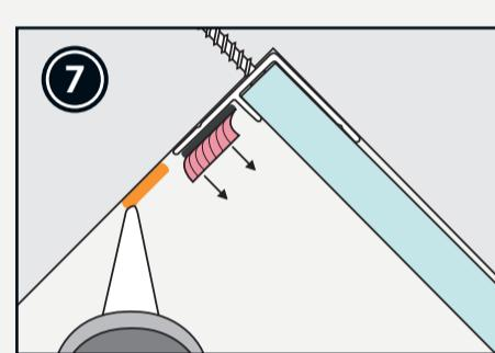
Place a bead of Fibo Seal on the left hand side of the corner profile. Remove protective tape cover on the corner profile before clicking in the last panel.
