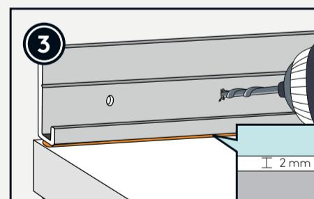
Fasten the bottom list to the back wall about 2 mm above the bench to make room for the sealant.
