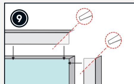
To cover the cut surfaces use an L-profile, cut to length and mitre the corner 45°.
