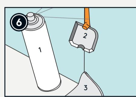
Excess sealant is easily removed by using Fibo Clean and Fibo Sealing Tools. Fibo Wipes can also be used, but soap residue from Fibo Wipes should be removed with paper and water to avoid stains.
