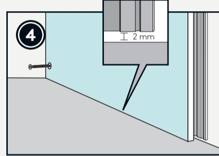
Keep 2-3 mm distance from worktop to bottom of panel. This gap will be filled with Fibo Seal.
