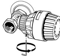
The clamping band can be rotated to one of four positions to allow easier access to the allen screw.
