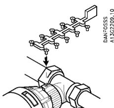
Push the theft protection device into the hexagonal hole of the allen screw.
