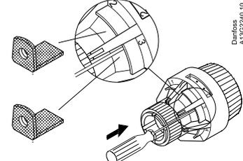
Example: Required locked value = "3" - Set thermostat at a setting below "3".
