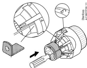
Example: Required max. value = "4" - Set thermostat at a setting below "4".
