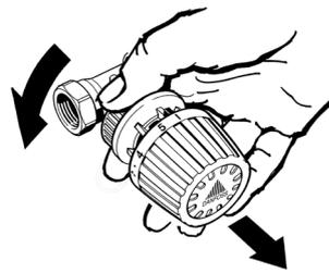
To remove the thermostat turn the base counter-clockwise. This will also reset the the snap-action mechanism when an audible "click" is heard.
