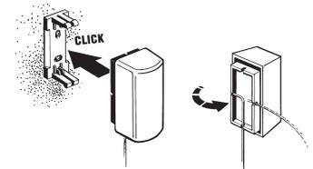
The remote sensor must not be in a drafty location or be covered. Do not install above a heat source. Attach the sensor bracket to the desired location. Pull out the required length of capillary tube and secure to the sensor as shown. Push the sensor onto the base.
