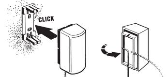
The remote sensor must not be in a drafty location or be covered. Do not install above a heat source. Attach the sensor bracket to the desired location. Pull out the required length of capillary tube and secure to the sensor as shown. Push the sensor onto the base.
