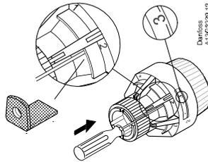
Example: Required min. value = "2" - Set thermostat at a setting above "2".
