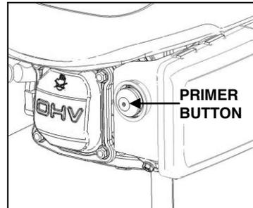
You also should put more fuel to mix air for easy start. When you push the primer button, it will pump the fuel direct from carburetor to burning house.
