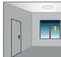
4. After elapse of stand-by period, the sensor switches off the light if no motion is detected in the detection zone.
