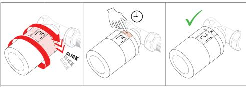
Screw the Danfoss  $Eco^{\mathbb{T}}$  onto the mounted adapter until a click sound appears. Once the thermostat is tightened properly, then adjust the display to your preferred display orientation. A large  $\widehat{m}$  is flashing in the display to indicate that Installation Mode is activated. Press and hold the button  $\widehat{\phantom{a}}$  for 3 seconds.
