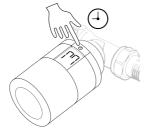
Press and hold until large fill flashes. This indicates you are in mounting mode
