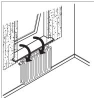
Danfoss Eco™ features an Open-window function, which closes the valve if the room temperature is falling dramatically, thus reducing the heat loss.
