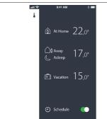
Scroll on temperatures to set your preferred temperatures. The Danfoss Eco™ can be set from 5°C to 28°C. Danfoss recommend a difference between 'At Home' temperature and 'Away/Asleep' that does not exceed 4 degrees.
