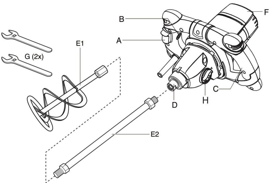
A Switch for on/off and speed control
