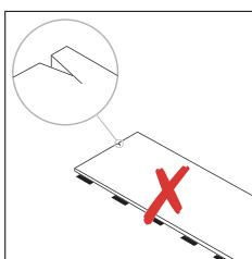
Cello Puzzle is not suitable for outdoor use or conservatories. Ensure that the indoor temperature is always kept above 5°C and ideally between 18 and 25°C.
