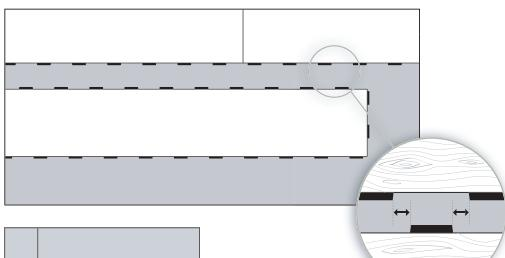
The click elements of the new row, need to be positioned, exactly in the middle of two locks of the previous row. From second row on, always connect the short side first and then the long side.
