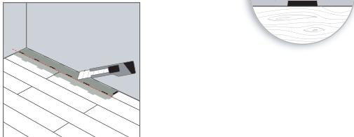
For door mouldings, lay a panel face down next to the door moulding. Saw the panel, then slide the plank under the moulding. Make sure the moulding doesn't support on the floor.
