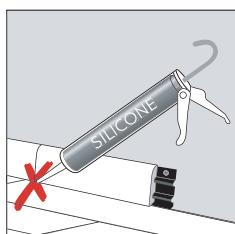
To allow the floating floor the necessary contraction and expansion we advise against fixing any accessory on the floor. Never attach skirting boards directly onto the installed floor. Permanent sealing products (silicone) should never be used to seal up the gap between the floor covering and skirting boards/profiles.
