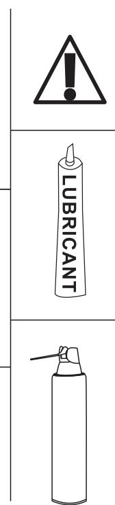
**GB** Grease or Lubricant oil must be applied onto the wheels and hinges after installation of the Product. For proper maintenance, shower wheels and hinges must be cleaned and lubricated every six months in order to function correctly. Use lubricant oil (such as "WD-40") or silicon spray.
