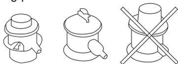
The 30 mbar low-pressure regulators in the picture are suitable for a gas barbecue, while the high-pressure regulator on the right is intended for LPG tools and must not be used with a gas barbecue.
