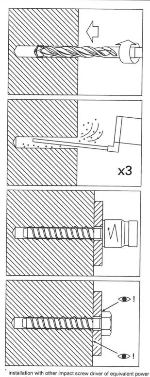
Drill hole with rotary percussive machine. Drill to a required depth.
