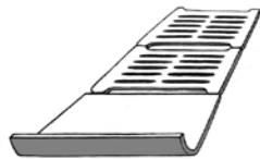
MACU stoves come with a cradle fireplace grate where a single wire tray grate is installed. An air iron plate is placed on the top shelf to direct the circulation of air in the upper part of the firebox. It is prohibited to use the stove without these parts. Note that these parts wear down over time and get bent and their form will change in use. You can purchase new ones as spare parts when needed (image on the right).
