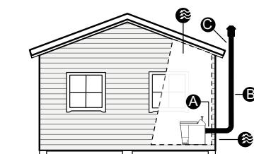
*NOTE! Only Ø110 mm vent.pipes made of plastic and 1pcs 90 ° bend may be used in the installation.*
