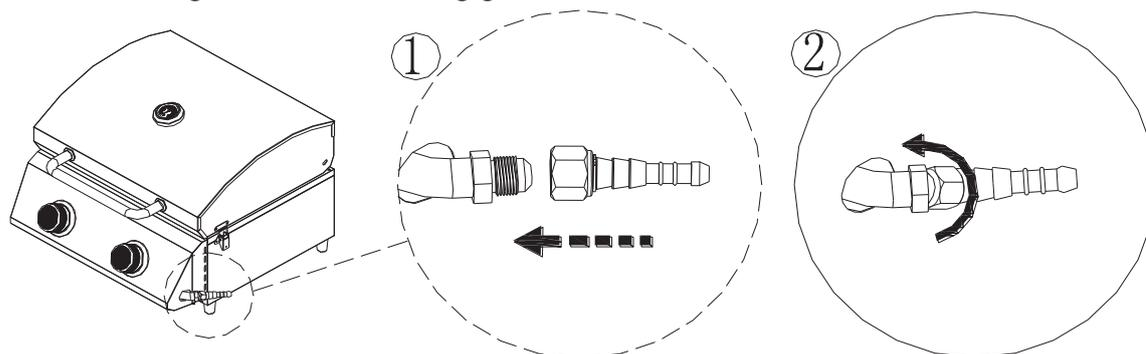
B: Assemble the gas regulator and hose for small gas bottle
