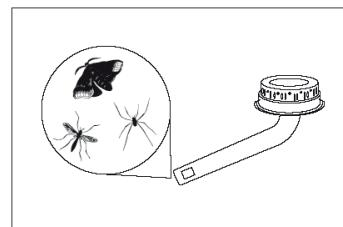
This may prevent gas from arriving to the venturi tube, causing yellowish, smoky flame at the burner or rendering lighting of the burner impossible. This could even result in combustion.
