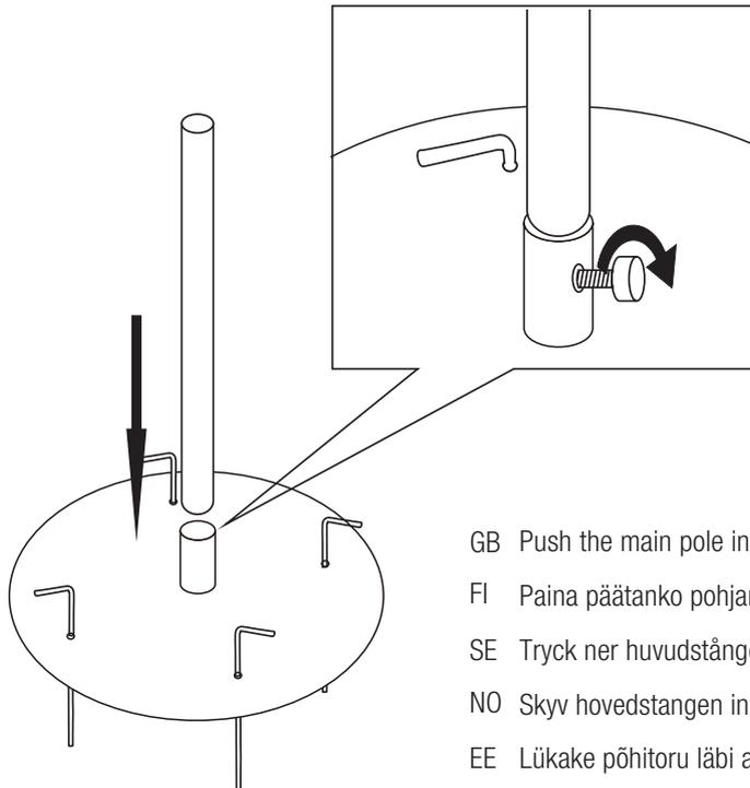
GB Push the main pole into the base hole, fix it by the big screw.
