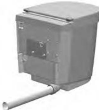
If the installation is to go through the floor, the pipe should be connected directly to the toilet, as shown below.
