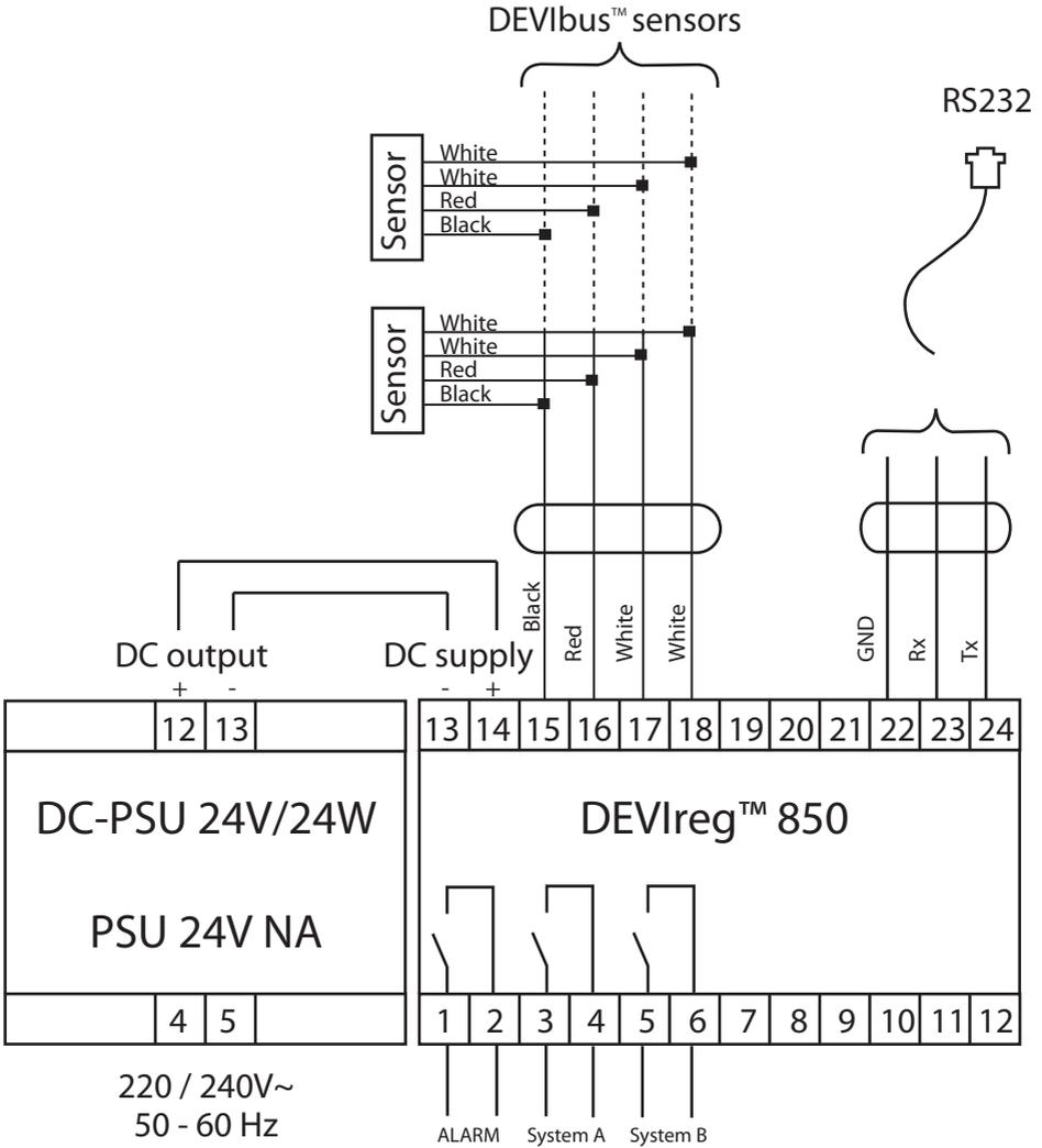
The DEVIreg™ 850 has an integral alarm function that monitors the attached sensors and the in-built microprocessor. An external alarm may also be connected to the system.
