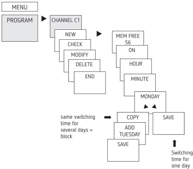
① A switching time always consists of a start time and an end time
