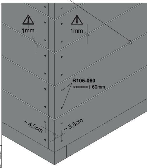
**EN** During the assembly of the planks it is essential to make sure that the planks are fixed with approx. 1mm distance and the top planks have the same height all around.
