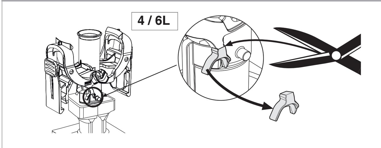
Water supply pipe connected to the left side
