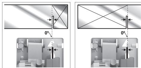
The cut mark (12) indicates the position of the saw blade when making a right-angled cut.
