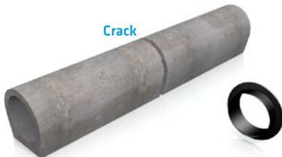
Remove damaged pipe section.
