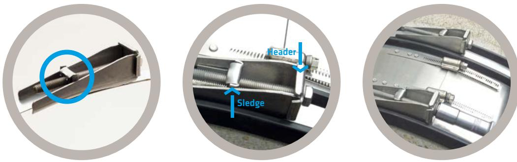
The purpose of this new development is to make the installation of the coupling to the pipe considerably quicker and much easier. The new bolting system has been engineered so that the sledge runs through the header casing, eliminating any protrusion of the bolt head.
