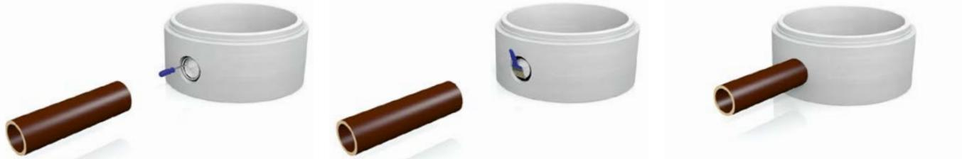
Remove polystyrene from socket.
