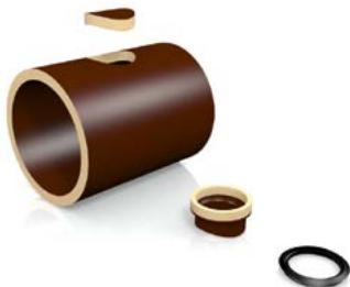
Drill and clean hole 90° to pipe axis.
