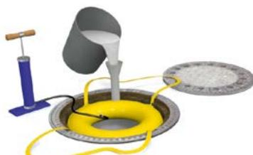
Blow up and position Shuttering-Kit. Then fill mortar into pour pipe.
