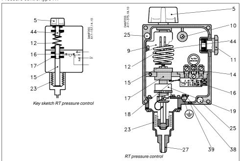
The bellows in the RT pressure control is connected to the low or high pressure side of the controlled system via the connection.
