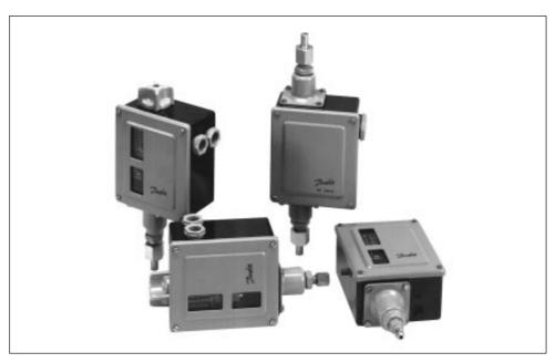
An RT pressure control contains a pressure operated single-pole changeover contact, the position of which depends on the pressure in the inlet connection and the set scale value. The RT series includes pressure controls for general applications within industrial and marine refrigeration.
