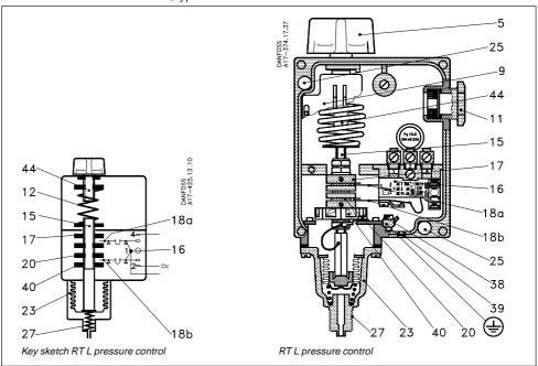
RT L pressure controls are fitted with a switch (17-4032) with an adjustable neutral zone. This enables the units to be used for floating control. The neutral zone switch contact arms (18a) and (18b) are operated by the spindle guide bushes (17) and (20).
