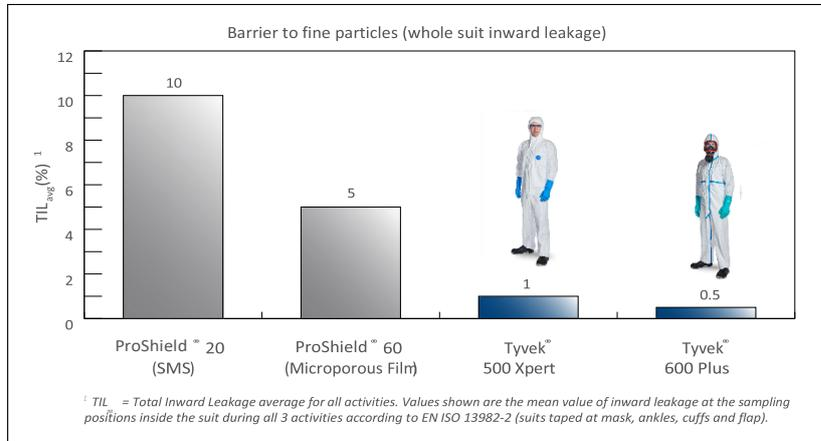
EN 1073-2\*\* measures the inward leakage of particles into the whole suit. The result is then expressed as the Nominal Protection Factor (NPF) of a garment. Tyvek® 600 Plus and Tyvek® 500 Xpert meet the requirements of Class 2 (NPF > 50), whereas most other Type 5 protective suits are only Class 1 (see table below).
