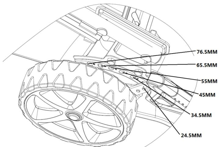
**! WARNING:** The blade can cause serious injury. Stop the engine before adjusting cutting height.
