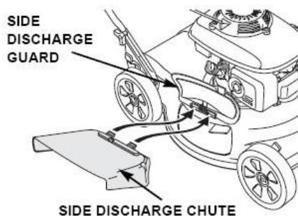
**Only Mulching:** Please remove the side discharge chute, close side discharge guard.
