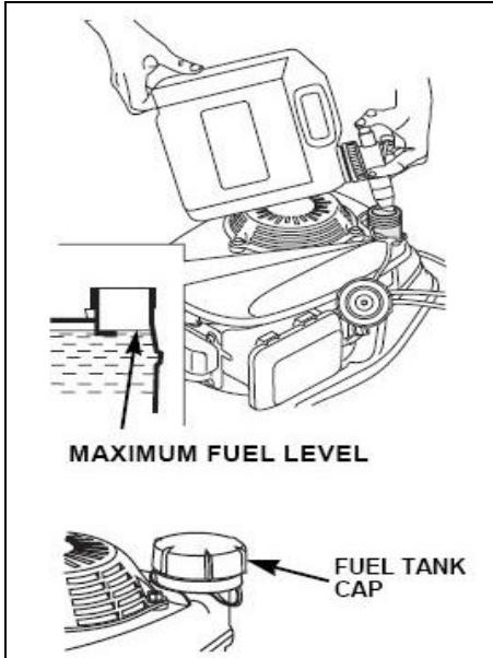
**! WARNING:** Gasoline is extremely flammable, and gasoline vapor can explode, causing serious injury or death. Use extreme care when handling gasoline. Keep out of reach of children.
