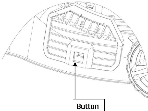
Press upward the button, then lift the side discharge guard, install the side discharge chute.
