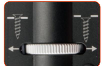
Before fastening on the deck top, drive a few screws into a scrap piece of material and adjust the depth set dial accordingly. For Face screws, you can drive them flush or countersink them.
