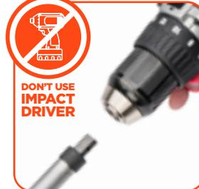
Make sure the drill is set in the forward position. Insert the large collar of the drive shaft into the drill chuck and tighten.
