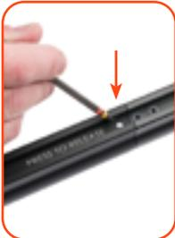
Using a bit, press the release button in the channel and remove the lower body of the tool.
