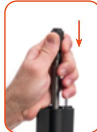
Put the T-15 bit in your other hand, pull down on the bit holder, and set the bit in place.
