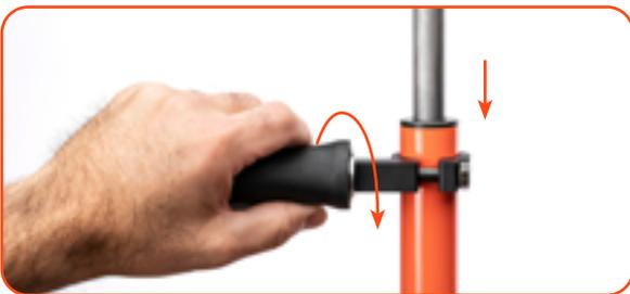
Loosen the handle by turning it counter-clockwise and slide the clamp onto the tool.
