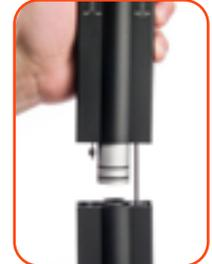
Slide the lower tool body over the bit—it will click into position.
