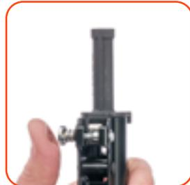
Insert the Face nose piece. It will lock into place.
