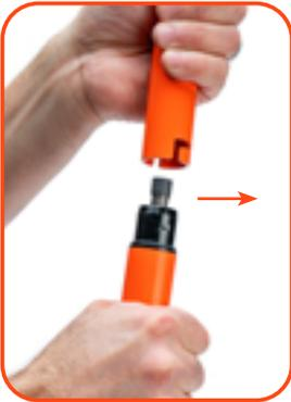
Separate the tool by turning the upper tool body counter-clockwise and sliding the locking pins out of the notches.
