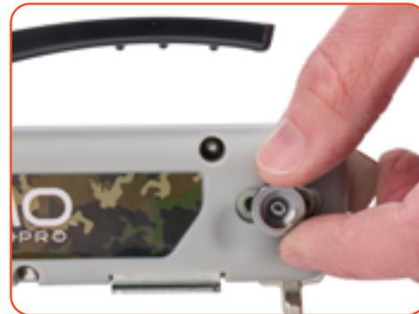
Adjust the spacer teeth on the tool with the thumb dial to fit your board.
