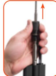
Pull up on the bit holder to ensure the bit is locked in.
