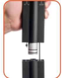
Slide the lower tool body over the bit—it will click into position.
