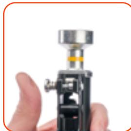
Insert the Clip nose piece. It will lock into place.
