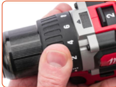
If your drill has a drill and clutch mode, set it to clutch mode. Set your drill to 30% of maximum torque.
