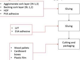
The manufacturing process of the flooring product begins by assembling the layers of agglomerate cork layer, backing cork layer and HDF, using a cold-melt adhesive. Then these components are blended with LVT, using a hot-melt adhesive. The resulting board is then cut into the defined dimensions and is now ready for packaging and storage.
