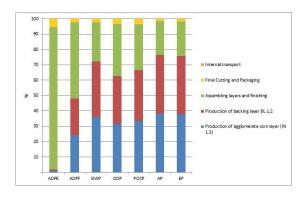
In the production of **Vinyl on Cork Flooring Floating**, the processes with the highest impacts are the production of the agglomerate cork layer, production of backing layer and assembling.
