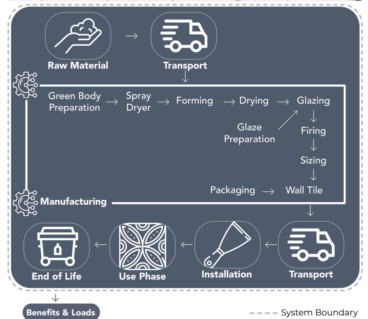
**A1:** Raw Material Supply includes raw material extraction and pre-treatment processes before production. For ceramic wall tiles, production starts with raw materials.
