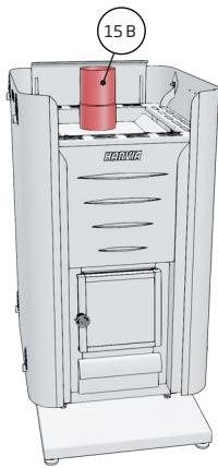
**GB** Install the smoke pipe in the outlet on top of the heater.
