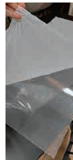
White protective film on the 4,0 mm roof panels indicates the UV protected side of the panel.
