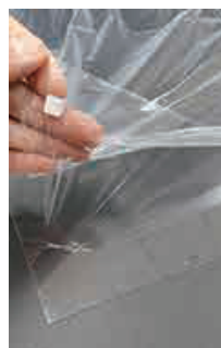
Transparent protective film on the 0,7 mm wall panels indicates the UV unprotected side of the panel.
