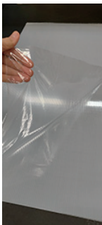
Transparent protective film on the 4,0 mm roof panels indicates the UV unprotected side of the panel.
