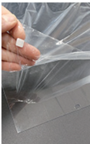
Transparent protective film on the 1,0 mm wall panels indicates the UV unprotected side of the panel.
