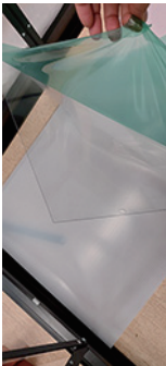
Green protective film on the 1,0 mm wall panels indicates the UV protected side of the panel.
