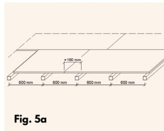
VMG Lignum Board | Floor are nailed or screwed. In service class 1, galvanize steel or stainless steel and in service class 2 - hot galvanized steel or stainless steel fasteners must be used. The minimum length of fasteners must be at least 50 mm or twice the thickness of the panel, whichever is the longest. For nails, the minimum diameter is 0.16 times the thickness of the panel; and 0.2 times the thickness of the the panel for screws. Minimal nails 3.0/50 mm, screws 3.6/50 mm.
