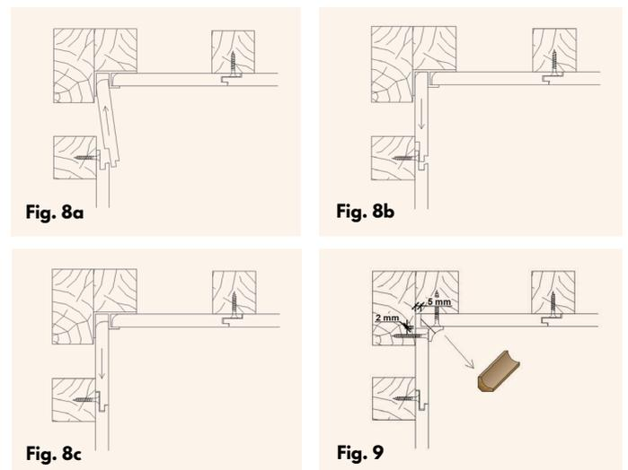
For external corners the first board should be cut 3mm in length, the final board – 10 mm. Edge of the board must be chamfer. The board marked with number 1 is installed first and then board marked with number 2.
