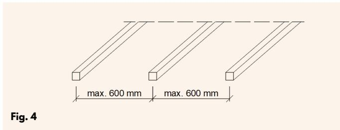
VMG Lignum Board | Floor should always be perpendicular to the direction of the beams (Fig. 5). All short panel edges must be supported. VMG Lignum Board | Floor must span at least 600 mm gaps, and connection must always be formed on the centre-line of a beam. In this case minimum distance from beam to joint should be 160 mm. If the short joints end up between the same pair of beams, the distance between the short joints must be the minimum 360 mm.
