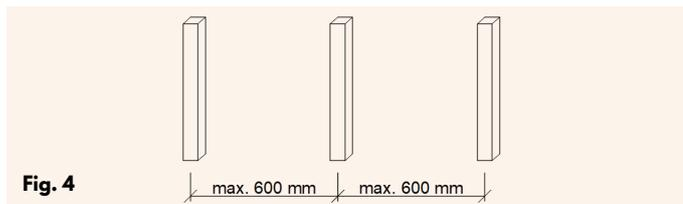
*VMG Lignum Board | Wall* are nailed or screwed. In service class 1, galvanize steel or stainless steel and in service class 2 - hot galvanized steel or stainless steel fasteners must be used.
