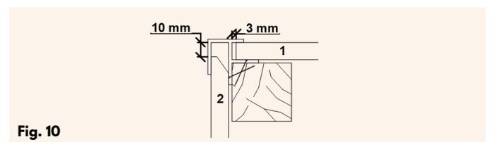
Against fixed structures, there must be a clearance of min. 10 mm (Fig. 11).
