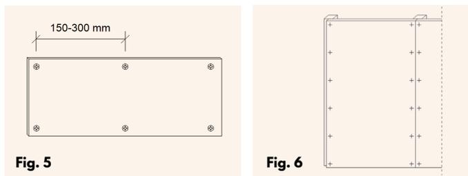
VMG Lignum Board | Wall T&G2 must be supported on 2 sides (Fig. 6). This support should be 18 mm at least (Fig. 8)
