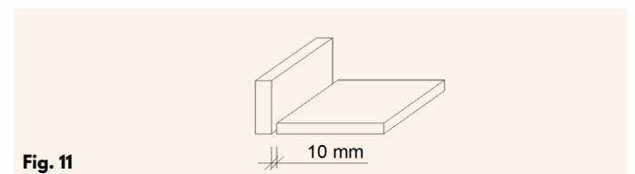
Before laying the top wall, it must be checked that the wall has good contact with the joists and does not creak. If it does, consider inserting more screws. VMG Lignum Board | Wall damp content may not exceed 10% when the top wall is laid.
