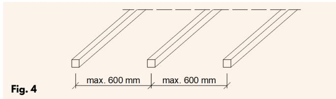
*VMG Lignum Board | Floor* should always be perpendicular to the direction of the beams (Fig. 5). All short panel edges must be supported. *VMG Lignum Board | Floor* must span at least two beam gaps, and connection must always be formed on the centre-line of a beam.
