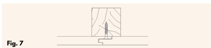
A corner fillet can be used on internal or external corners. Corner fillets must be installed before mounting boards. The installation instructions for internal corners are given in Fig. 8a, 8b, 8c and Fig. 9, for external corners Fig. 10. For internal corners chamber the back edge of the board. The board should be guided into base of fillet (Fig. 8a) and then pressed towards the wall (Fig. 8b). And then the board should be pulled back, engaging the tongue and groove (Fig. 8c).
