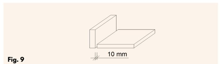
Before laying the top floor, it must be checked that the subfloor has good contact with the joists and does not creak. If it does, consider inserting more screws. VMG Lignum Board | Floor damp content may not exceed 10% when the top floor is laid.
