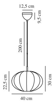
Voltage (V): 220-240 Volt IP degree: IP20 Maximum bulb wattage (W): 40W Class (Class 1, Class 2, Class 3): Class 2 (Double isolated) Socket type: E27 Parallel connection: False
