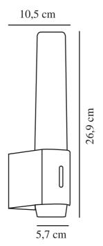
Voltage (V): 230 Volt IP degree: IP44 Class (Class 1, Class 2, Class 3): Class 2 (Double isolated) Socket type: LED Module
