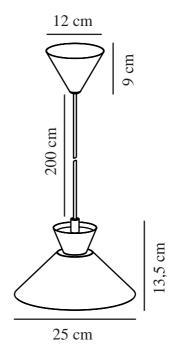
Voltage (V): 220-240 Volt IP degree: IP20 Maximum bulb wattage (W): 40W Class (Class 1, Class 2, Class 3): Class 2 (Double isolated) Socket type: E27 Parallel connection: False
