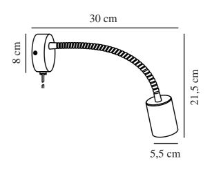
Voltage (V): 220-240 Volt IP degree: IP20
