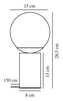
Voltage (V): 220-240 Volt IP degree: IP20 Maximum bulb wattage (W):
