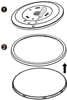
1. Remove the diffuser and light guide plate.
