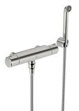
Thermostatic shower faucet. Bidetta hand shower, shower hose and wall bracket. Temperature handle equipped with safety stop at 38°C. Volume handle with EcoFlow control. The faucet includes vacuum breaker, litter filters and non-return valves.
