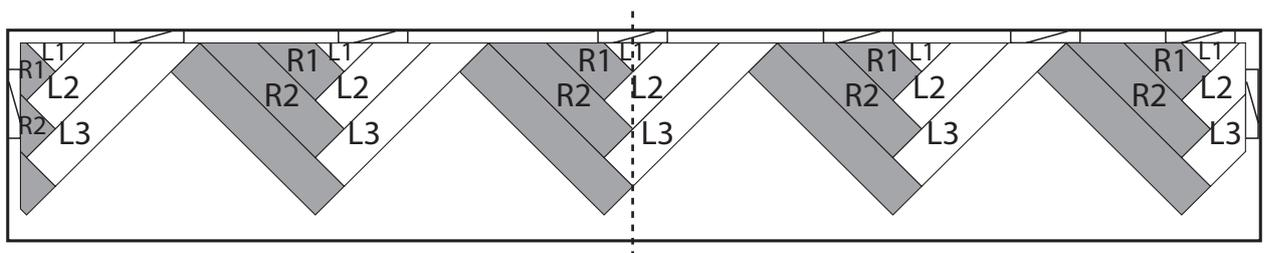
Always make sure that you make perfect angles of 90°. If you notice that a long or short side does not join well, this is because the legs of the herringbone are too 'wide' or too 'narrow'. Tap a piece of leftover board with a plastic mallet until the connection joins neatly and only then continue laying. If you do not do this at the start you will have problems later during laying. Starting again is then the only solution.
