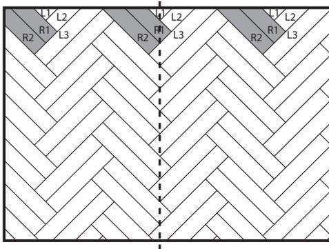
**1** Thoroughly clean the floor and open different packages. Keep the left and right-hand boards well separated, and lay them ready with the groove on the long side facing you.
