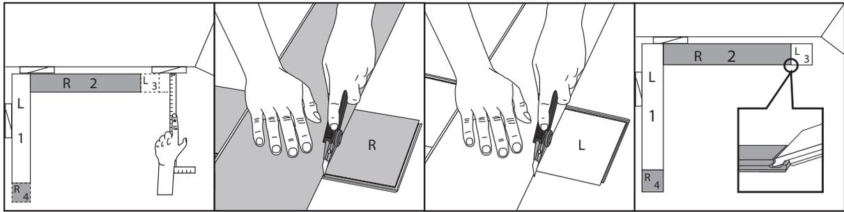
**11** If you have to work around pipes, ideally make sure that the pipe is at the meeting point between two planks. You can then work neatly around the pipe while keeping the 8 mm expansion space all around. If the pipe falls unavoidably in the middle of a plank, you will have to saw a piece out of the plank. Trim this piece to allow space for the pipe then replace it, possibly with a little adhesive to keep it in place.
