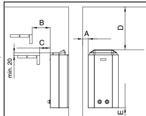
Figure 1. Minimal safety clearances for the heater.
