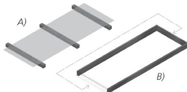
6. Lift the frame in position according to the desired handedness. Screw lightly the topmost screws on both lock and hinge side.
