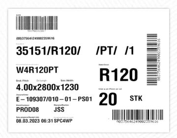
Each board on the bottom has a production batch code. One should use boards from same production batch for installation.
