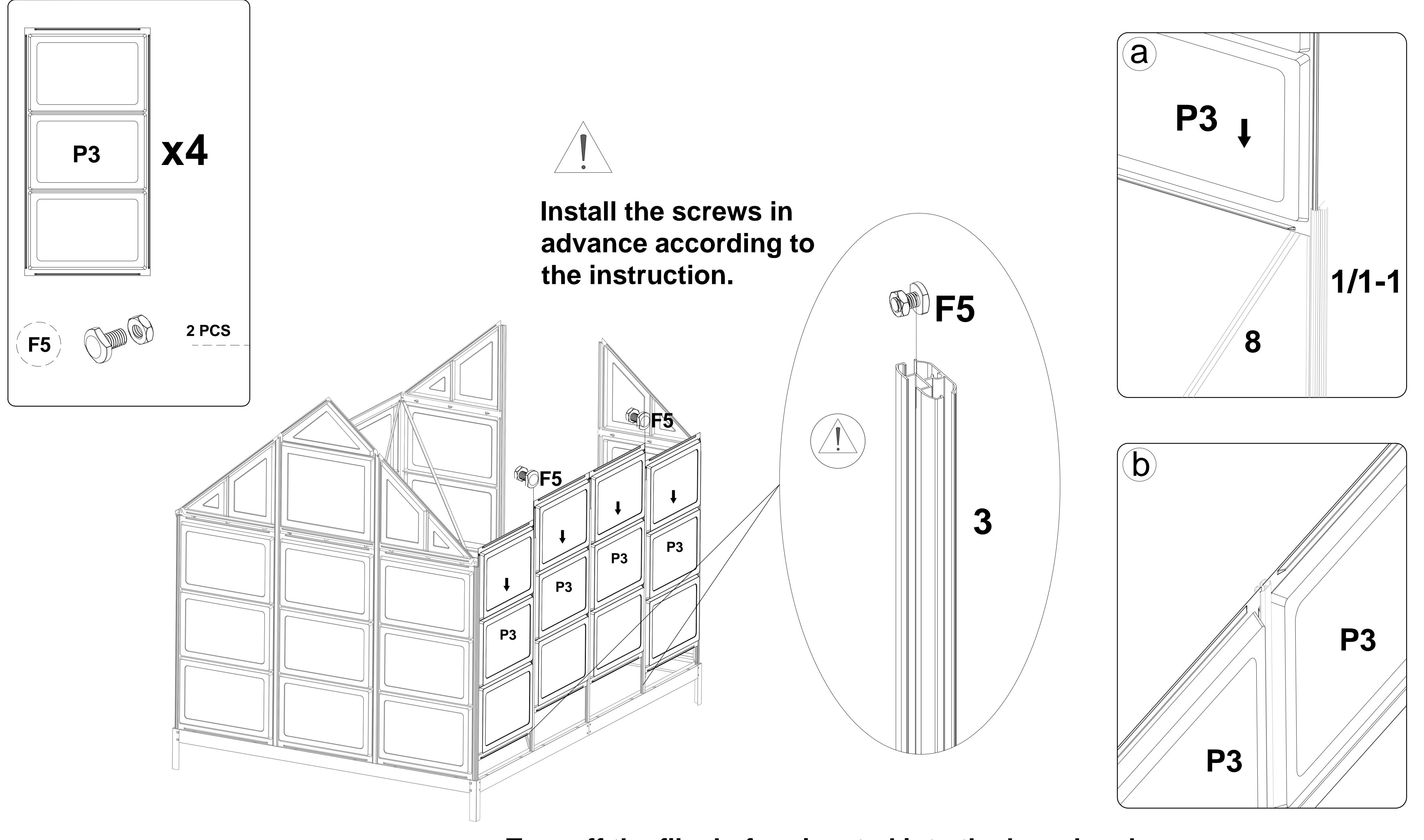
Tear off the film before inseted into the board and the side of white film needs faced out.
