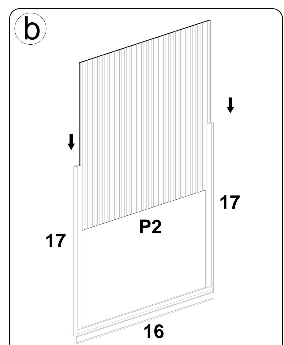
Tear off the film before inseted into the board and the side of white film needs faced out.
