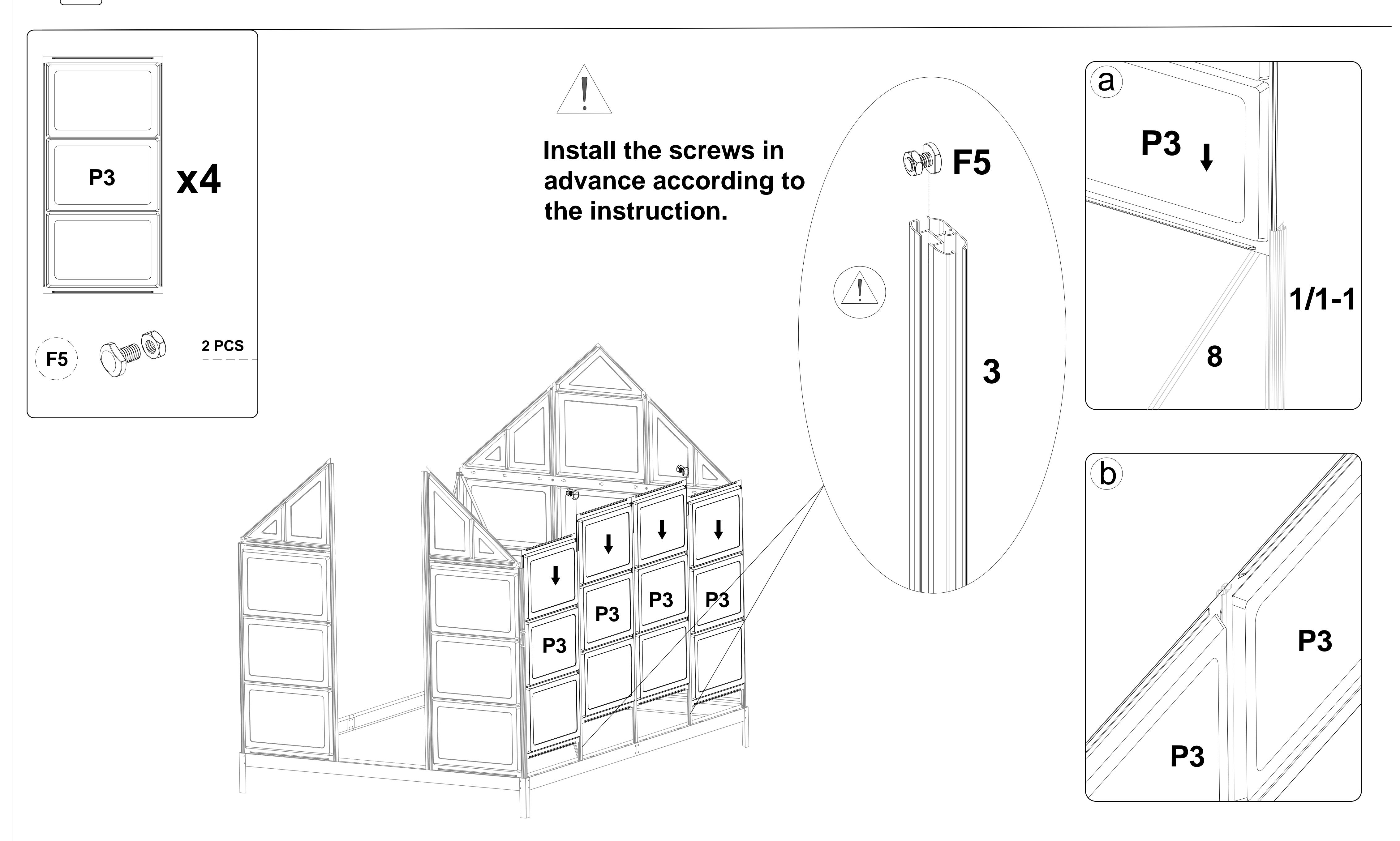
Tear off the film before inseted into the board and the side of white film needs faced out.
